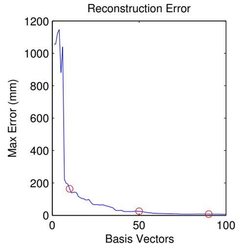
**Figure 7:** The maximum position error (over all frames and markers) for reconstruction from a given number of SVD basis vectors. Red-circled errors correspond to the frames shown in Figure 1.
