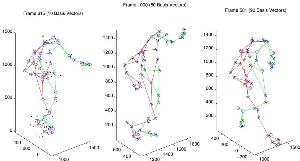
**Figure 1:** Representing a set of motion capture markers by the all-pairs distances between them allows for ludicrously good compression with low error. These are the frames containing the maximum positional error for different numbers of retained basis vectors (circled in Figure 7). Reconstructed positions are shown as circles, and the real positions are shown as dots. Ideally, every dot should be in the center of a circle.
